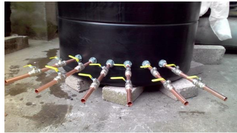
Rainfall Simulator 2 No. 1250l water tanks Manually adjustable valve controls To mimic any storm event At full plot scale
